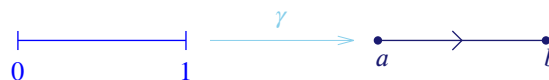
Figure 9.2: A parametrized curve \gamma : [0, 1] \subset \mathbb{R} \rightarrow \mathbb{C} , \gamma(t) = a + t(b - a) .
